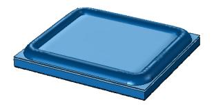
Finally, mounting a membrane and a plate closes the acoustic shortcut and increase the effective area, thus enabling the sound generation.
